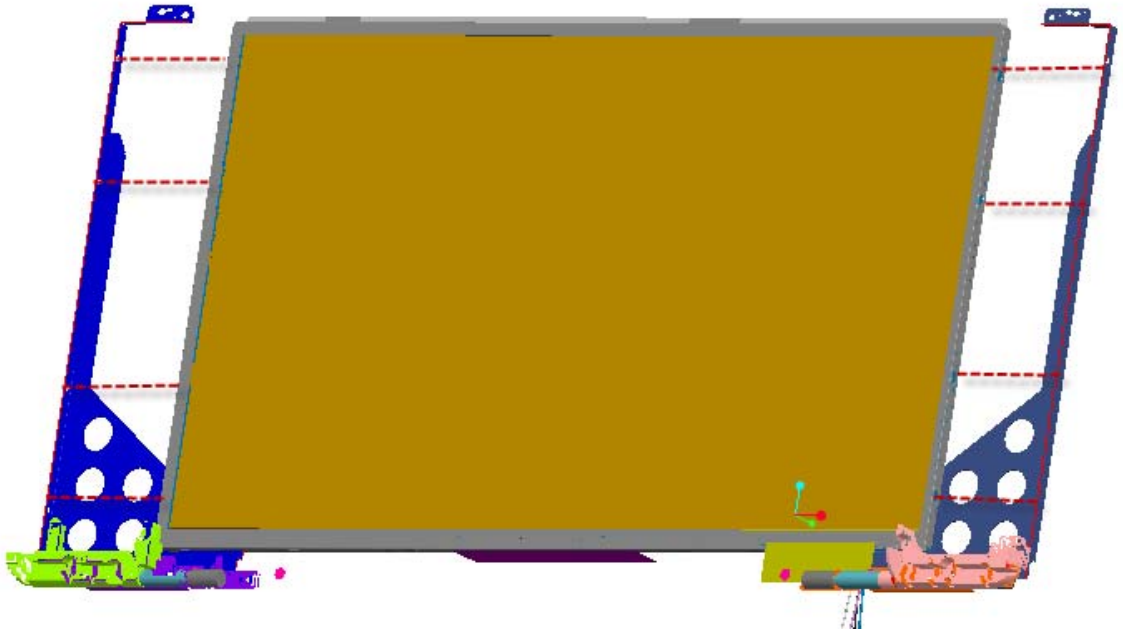
Figure 4-16-4 Remove the LCD hinge
